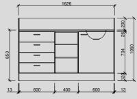
• overall width: 1626 mm • modules: drawer module, large shelves and wash basin module with door
